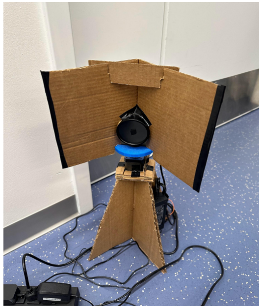
Figure 2.3: Photograph of Infrared Beacon
